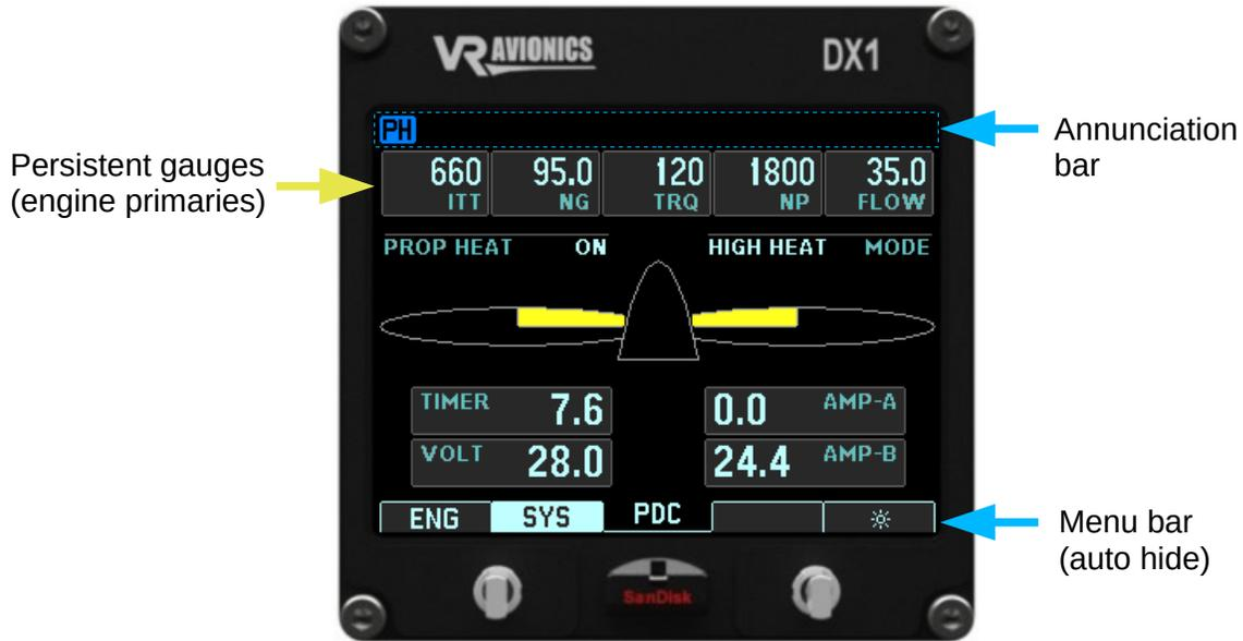
Except for the Annunciation bar and persistent gauge stack at the top and the Menu bar at bottom, this page shows information relating to the PDC (propeller heating) system.
