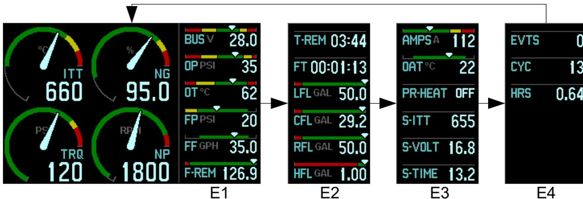
The readings in E1 through E4 depends on the information the installed LRU's provide. Some measurements have redundancy with two or more LRU's providing the same parameter (eg. N1). In such cases there is a preferred source, but should this source become unavailable the display will automatically switch to the next alternative in line, and so forth.
