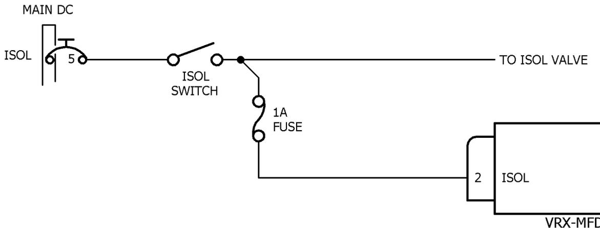
To include this feature the circuit above must be wired-in. A small fuse (or ½ watt 10KΩ resistor) should be installed as indicated very close to the ISOL switch. This ensures no short in the line from the fuse to pin 2 on the MFD can hamper activation of the ISOL circuit.
