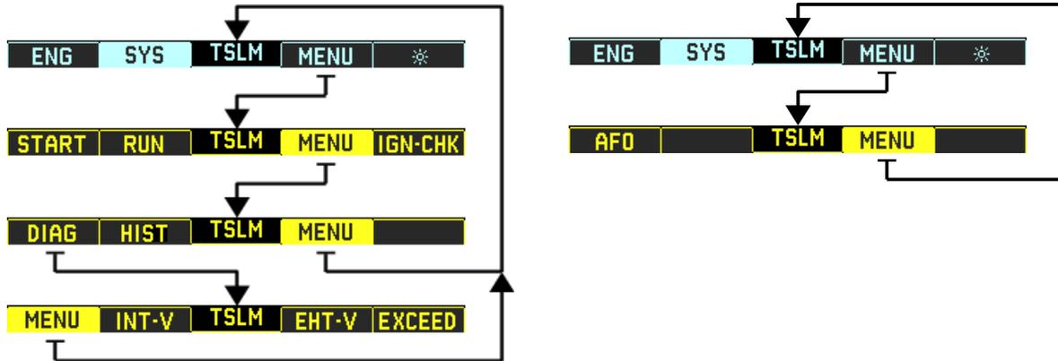
The menu structure on the left will show if the engine is **not** running, and the one on the right if it is running. The menu allows the following TSLM operations:
