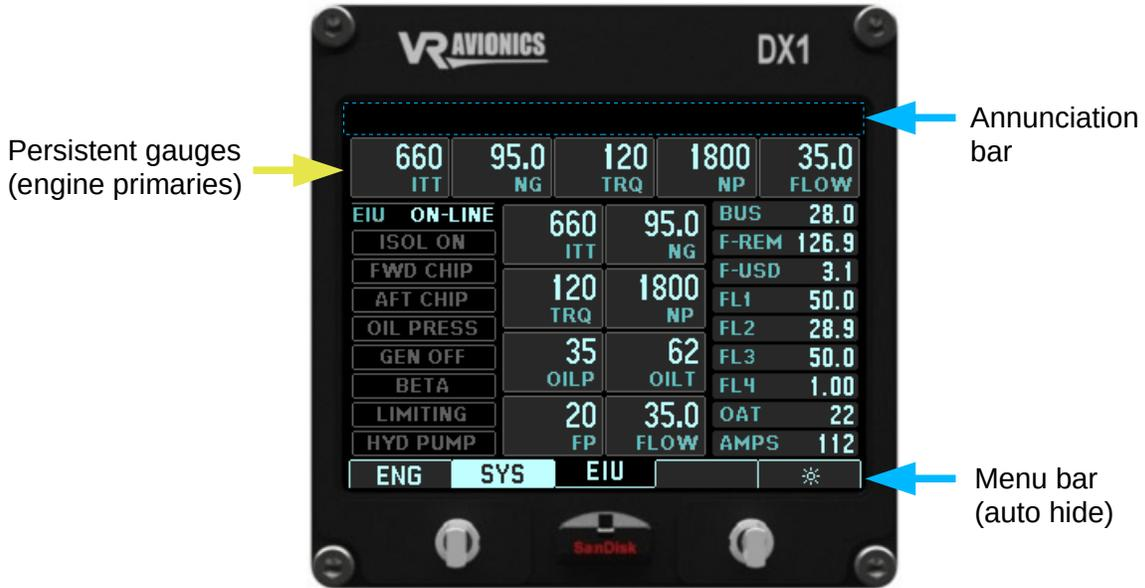
Except for the Annunciation bar and persistent gauge stack at the top and the Menu bar at bottom, this page shows information relating to the EIU monitoring system:
