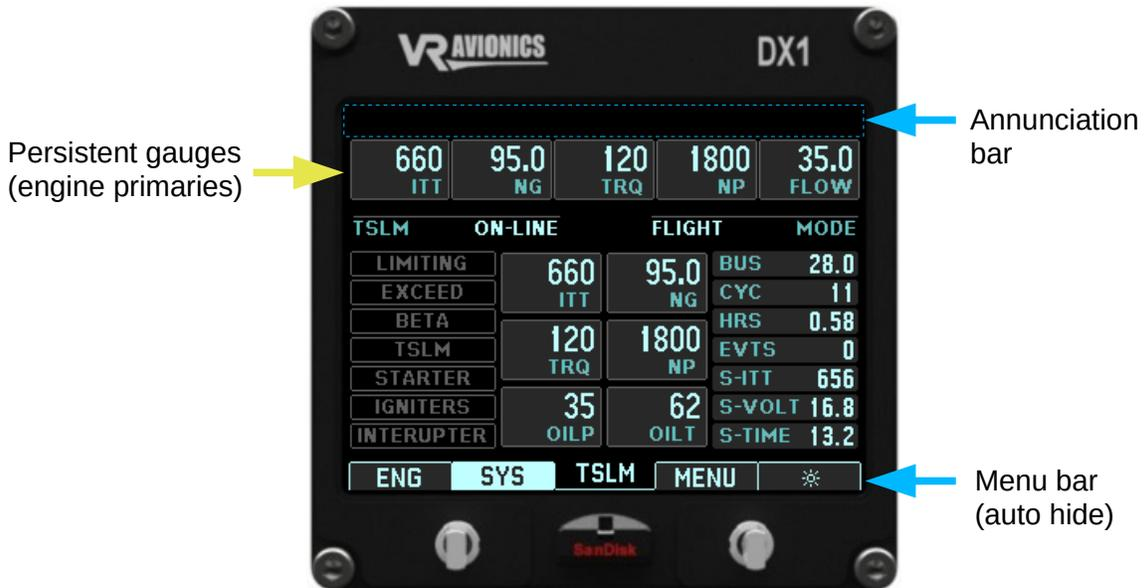
Except for the Annunciation bar and persistent gauge stack at the top and the Menu bar at bottom, this page shows information relating to the TSLM system:
