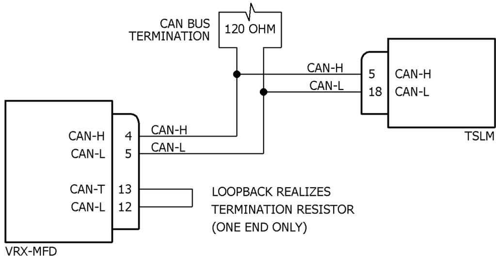
If the total length of the CAN bus cable that connects everything is short enough (under 2 meters) as the case may be in the above example the remaining 120 ohm termination resistor may be omitted.
