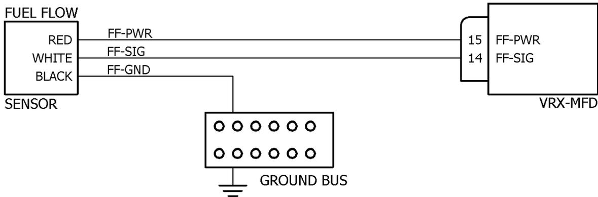
Any pulse based fuel flow sensor, where the output frequency linearly represents the rate of flow, may be used. For the Walter M601 we usually recommend the FT-180 (black cube) from Electronics International ([www.buy-ei.com](http://www.buy-ei.com)).
