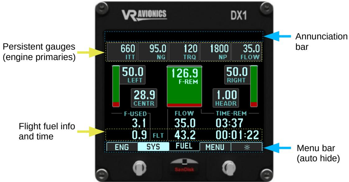
It shows the Annunciation bar at the top and the Menu bar at the bottom. A stack of gauges persistent to all system pages lies just below the Annunciation bar. The rest is filled with the following info:
