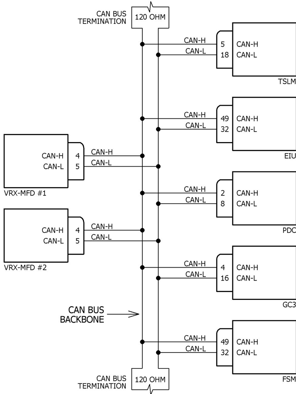
Splicing of the CAN-H (high) and CAN-L (low) wires should preferably be done inside the connector back-shell of each unit.
