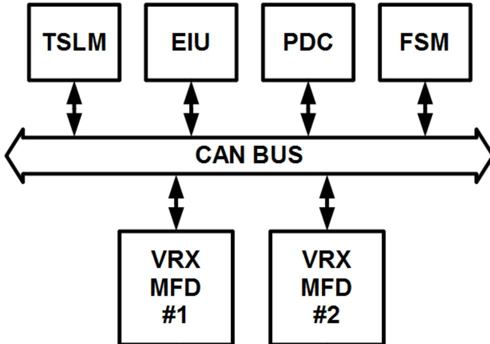
The different LRU's operate independently, though when combined as illustrated the user gains new capabilities and closer interaction. The standalone LRU's have separate manuals describing their installation and operation, and should be used in conjunction with this manual. They may be downloaded from the VR Avionics website.
