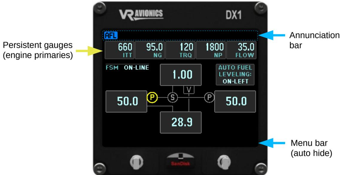
Except for the Annunciation bar and persistent gauge stack at the top and the Menu bar at bottom, this page shows information relating to the FSM system.
